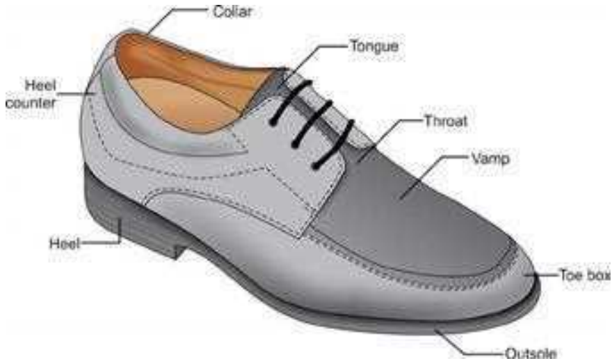
Fig. 12.8: Parts of footwear.
