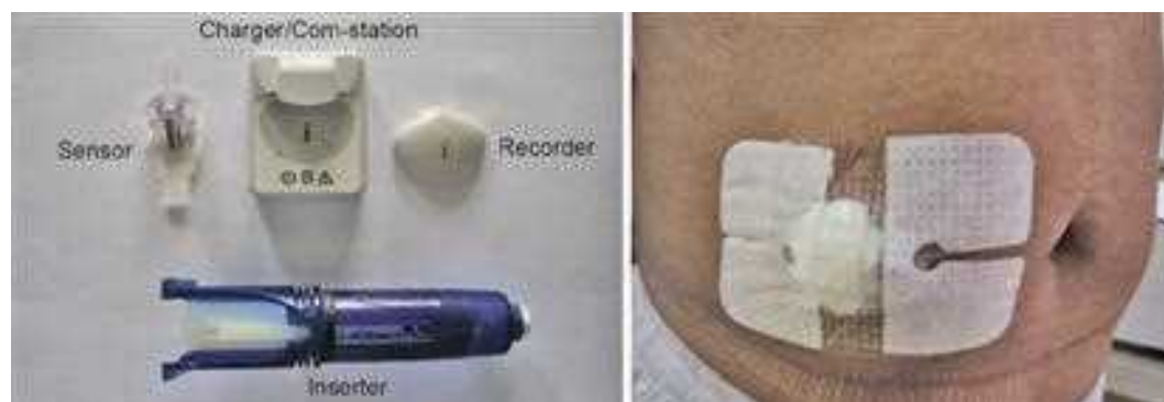
Fig. 9.4: Newer continuous glucose monitoring system (CGMS) devices collect glucose data and send the data wirelessly to the monitor for real time use or the data can be downloaded to the computer for analysis.
