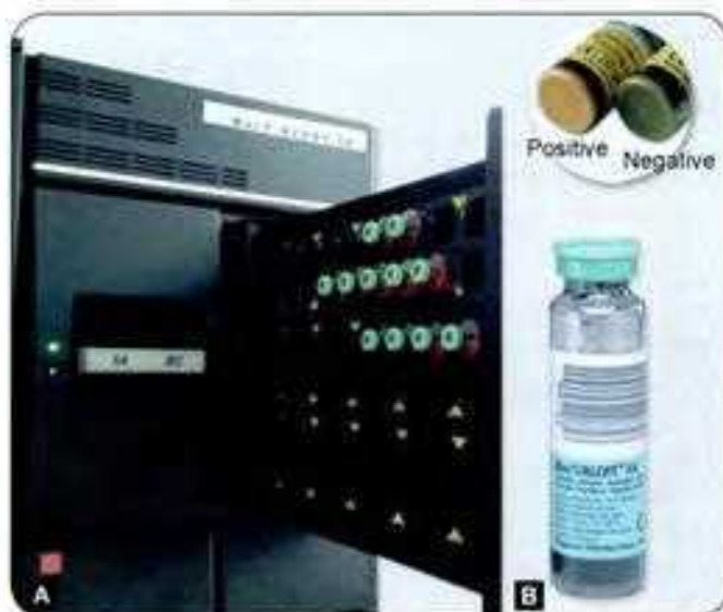
Figs 5.9A and B: A. BacT/ALERT automated blood culture system; B. BacT/ALERT blood culture bottle
