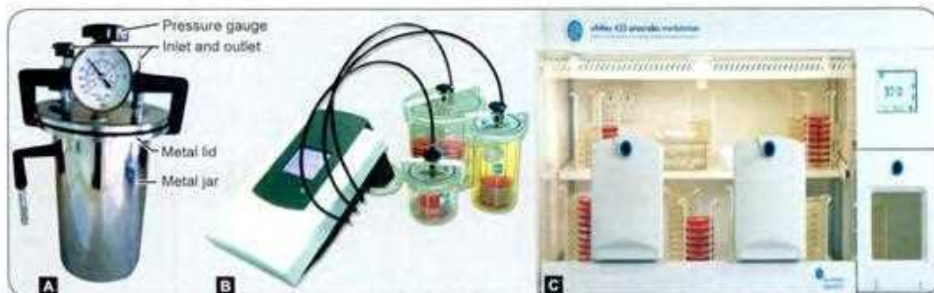
Figs 4.12A to C: A. McIntosh and Filde's anaerobic jar; B. Anoxomat anaerobic system; C. Anaerobic work station (Whitley pvt. Ltd.)
