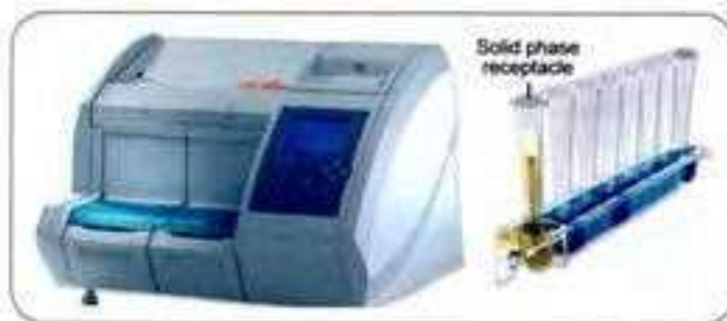
Fig. 12.19: miniVIDAS system and reagent strip (first well is solid phase receptacle coated with Ag or Ab and other wells contain various reagents)
