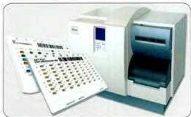
Fig 5.12: VITEK 2 system with its panels (reagent cards) for identification and antimicrobial susceptibility test
