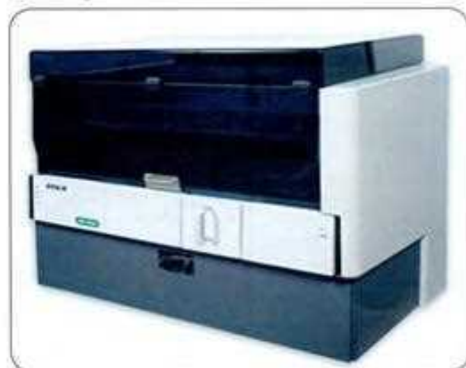
Fig. 12.12: Automated ELISA (EVOLIS System, Biorad) Source: Department of Microbiology, JIPMER, Puducherry (with permission).
