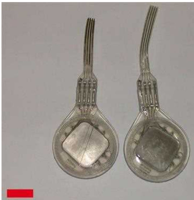
Fig. 11.24 These electrical transducers with wires running to the low chest served to stimulate the diaphragms. An external electrical stimulator device produced electrical activity in these receivers
