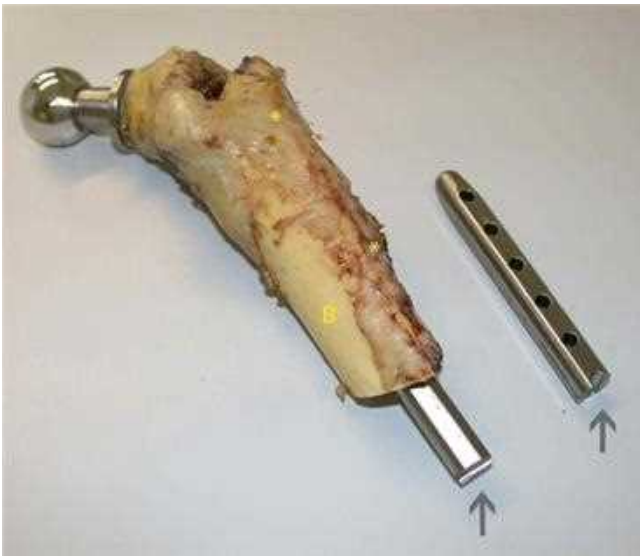
Fig. 11.57 This complicated hip fracture needed a metal prosthesis and reinforcement with allograft bone and cement ( asterisk ). Whilst this procedure was a success with regard to allowing incorporation into native bone ( B ), the metal device failed, with fracture of the metal stem adjacent to a drilled hole ( arrow )
