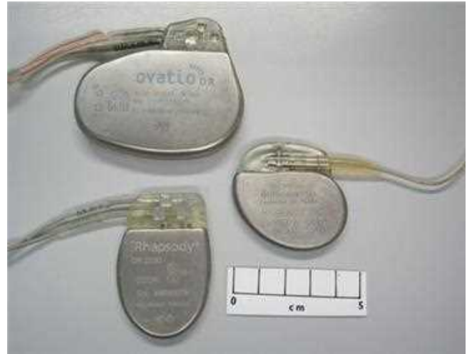
Fig. 11.28 A range of cardiac pacemakers: The modern variety have a smooth external case, with the manufacturer's data and serial numbers. Leads emerge from one point on the device and pass onwards to the heart. At autopsy, most cases have the generator unit ( box ) cut free from the wires to allow easy extraction. If the device may have not worked adequately, the entire unit with wires and electrodes needs to be retrieved intact and sent for specialized analysis
