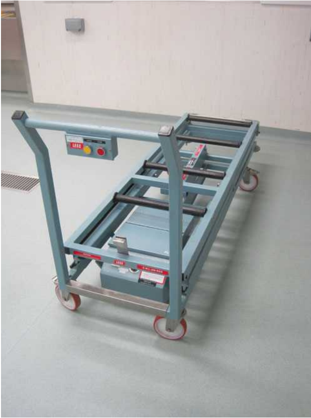
Fig. 1.18 Moving bodies around in the mortuary requires safe working practices to avoid mortuary staff injury. Here a hydraulic unit is employed to allow the fridge tray and body to be moved safely to the operating station
