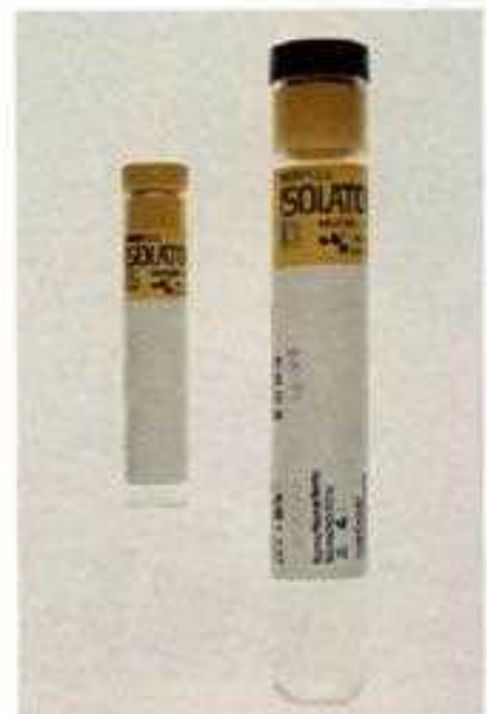
2-12 Isolator lysis-centrifugation blood culture system, 1.5 and 10-ml tubes (Wampole Laboratories, Cranbury, N.J.) are recommended for the isolation of mycobacteria and fungi. The tube contains a blood cell lysing fluid of saponin, polypropylene, SPS, fluorinert, and EDTA. Specimens collected in the 10-ml tube are centrifuged at 3000 \times g for 30 minutes. The supernatant is discarded, and the sediment is plated onto selected media. Specimens collected in the 1.5 ml tube are plated directly onto media.
