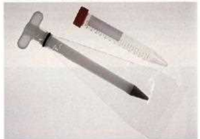
3-13 Another method for homogenizing tissue is using a disposable tissue-grinding kit (Sage Products, Cary, Ill.). This system minimizes contamination and splattering of the specimen.
