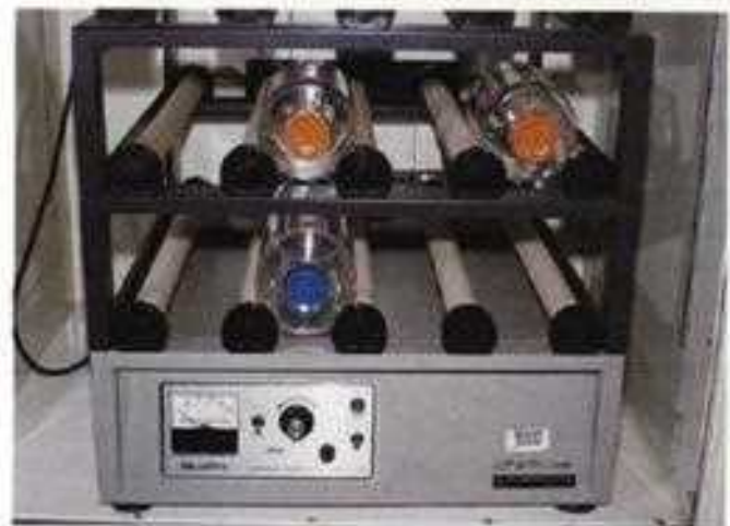
16-9, 10 Roller bottles. Roller bottles are also utilized for growing large quantities of viruses in cell monolayers (Figure 16-9). The cells are seeded into the bottle with medium and the bottles are placed in a roller bottle apparatus (Figure 16-10) located inside an incubator that continuously rotates the bottles. Once the cells are attached in a monolayer around the interior walls of the bottle, the viral inoculum is added and the bottle placed back on the rotating module (New Brunswick Scientific, Edison, N. J.). The cells can be harvested when the desired CPE is observed in the cell monolayer.
