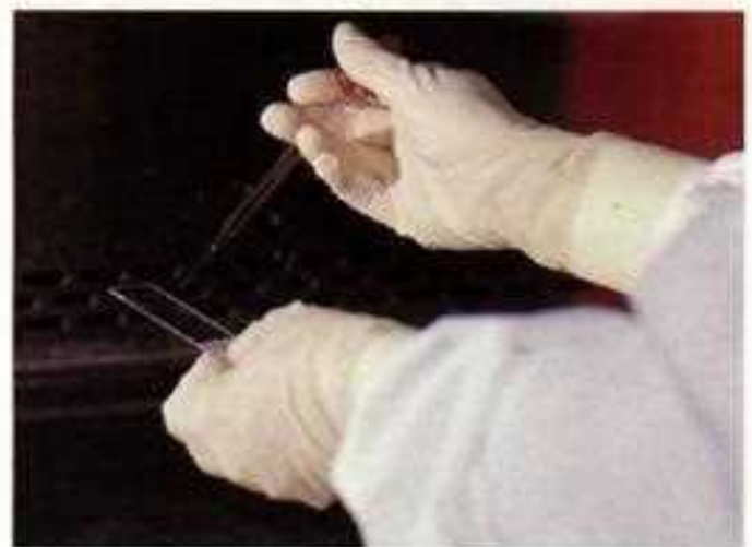
3-21 When a sterile Pasteur pipette is used to inoculate fluids onto a slide, enough specimen must be placed on the slide to form a circle of approximately 15 mm in diameter. The slide should air dry in the biological safety cabinet before it is fixed and stained.
