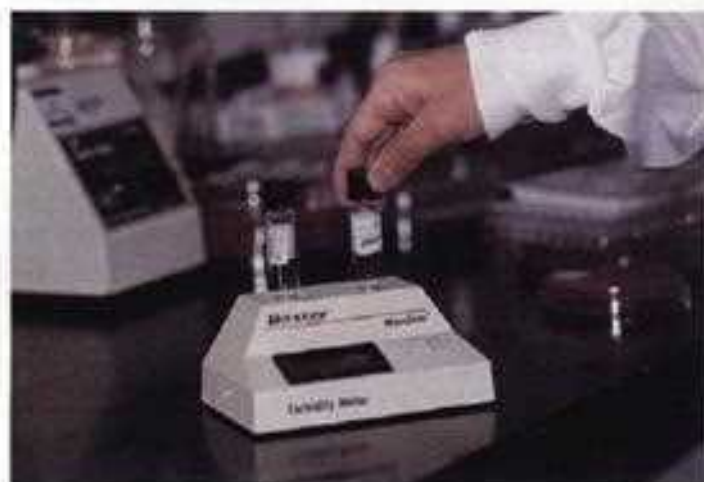
13-2 Using a turbidity meter to adjust the inoculum. The suspension is vortex mixed for 15 to 20 seconds before determining its turbidity. A meter is used to adjust the inoculum to a 0.5 McFarland turbidity standard, which is equal to approximately 1.5 \times 10^8 colony forming units (CFU) per ml. The turbidity is adjusted to match the standard by diluting with additional saline or broth.
