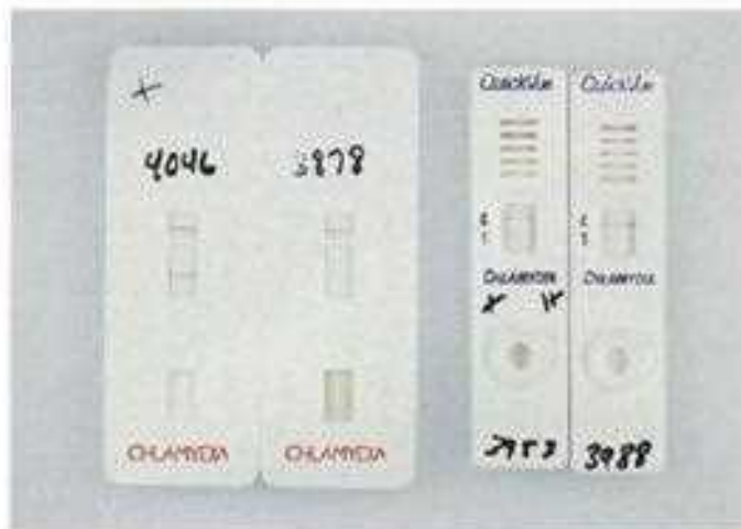
12-4 Chlamydia trachomatis . Direct antigen detection. There are several commercially available filter-based enzyme immunoassay systems for the direct detection of C. trachomatis . For each of the two assays depicted here, the specimen is placed in the lower window of the card. The antigen migrates through the filter and binds to a chlamydial-specific antibody located on a line in the filter at the level of the second window. A positive reaction results in the formation of a color line (see cards on the left side for each system). Another antibody located in the filter at a greater distance from the specimen window is used as a control to ensure that the specimen has migrated through the filter.
