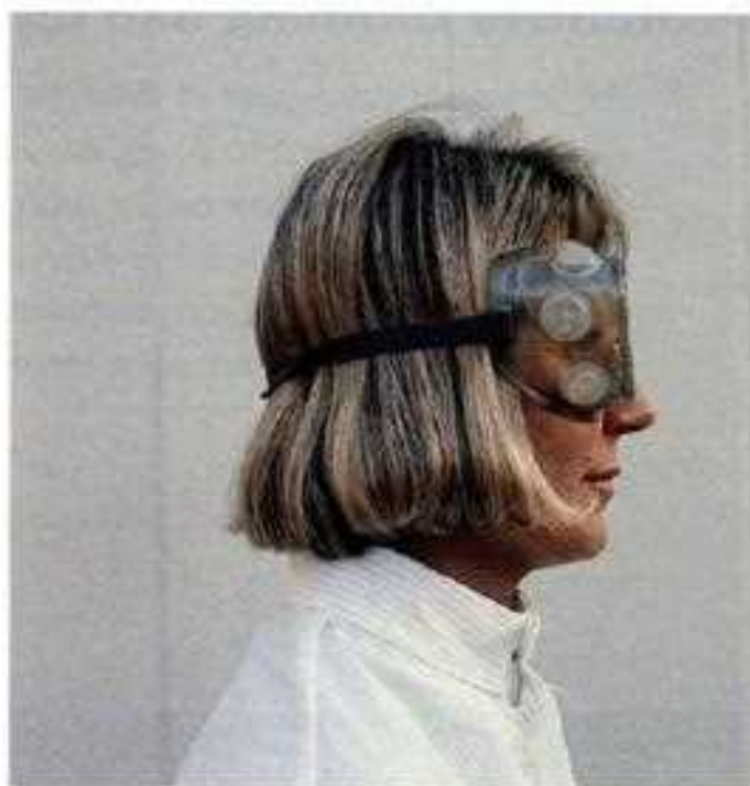
1-6 Eye covering such as goggles should be worn whenever working with body fluids or other specimens that may splash or procedures that may create aerosols. Goggles with side panels should be provided for each worker.
