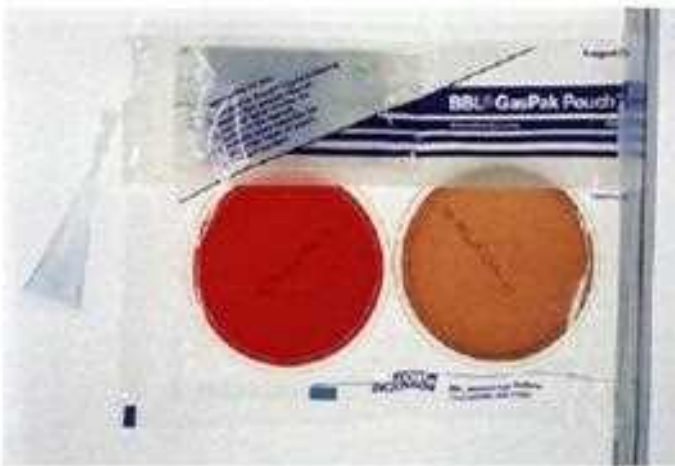
3-34 The GasPak anaerobic pouch (Becton Dickinson Microbiology Systems, Cockeysville, Md.) is based on the same principle. The bag is oxygen impermeable, and the system contains its own gas-generating kit and cold catalyst.
