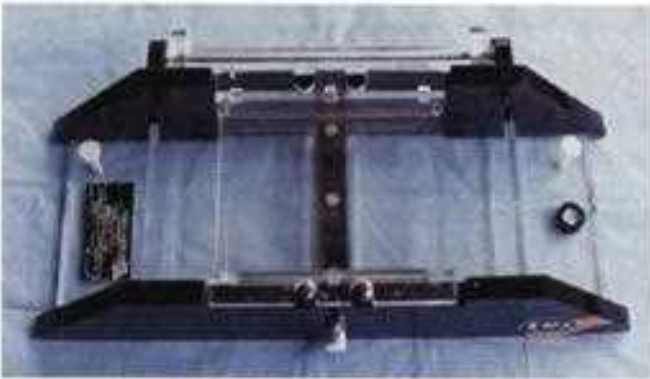
18-4 Gel apparatus (International Biotechnology, Inc., New Haven, Conn.). Restriction fragment length polymorphism (RFLP) analysis allows for the detection of genetic differences between organisms. Restriction endonucleases are enzymes that recognize, bind and cleave specific DNA sequences. When the DNA of different organisms is digested with these restriction enzymes, fragments of different sizes may result. After enzyme treatment, DNA fragments are separated on a gel apparatus.
