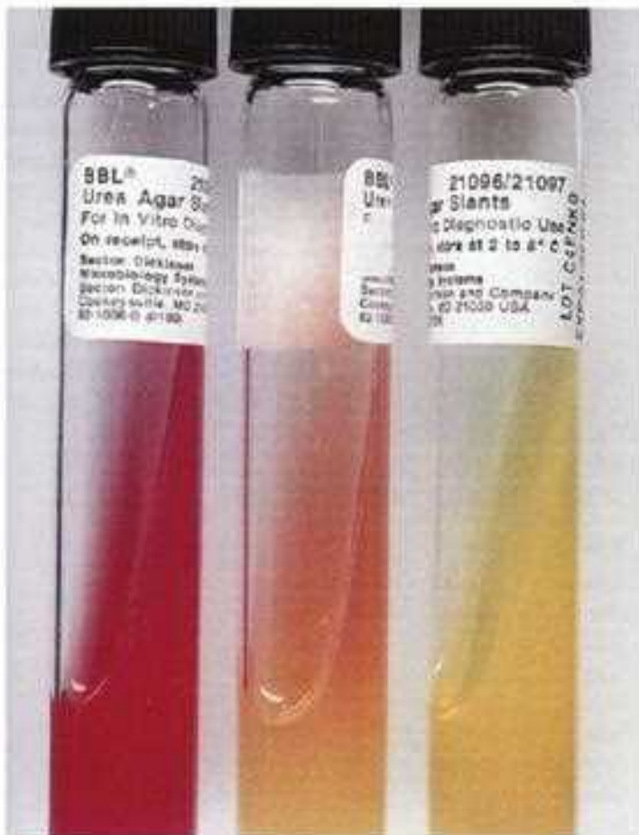
B-16 Urease test. Microorganisms that possess the enzyme urease hydrolyze urea to ammonia and \text{CO}_2 . The phenol red indicator turns cerise (dark pink) in the presence of the alkaline end products. This figure shows three inoculated Christensen's urea slants that were incubated overnight. The left and middle tubes are positive. The left tube was inoculated with Proteus mirabilis , a rapid urea hydrolyzer (2 to 4 hours), the middle tube was inoculated with Klebsiella pneumoniae , a slow urea hydrolyzer (18 to 24 hours), and the right tube was inoculated with E. coli , a urease-negative microorganism.
