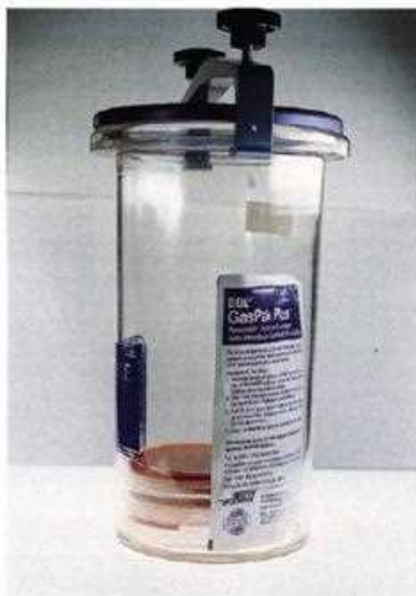
3-33 The GasPak anaerobic jar system (Becton Dickinson Microbiology Systems, Cockeysville, Md.) contains a hydrogen and CO 2 generator envelope, a disposable methylene blue indicator, and a catalyst basket in the lid.
