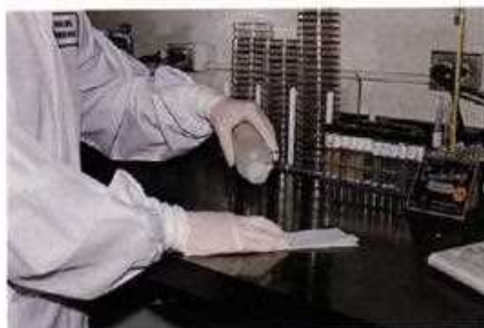
1-14 Decontamination of work surfaces at the end of each shift and cleaning of spills should be performed with a fresh 10% solution of household bleach.
