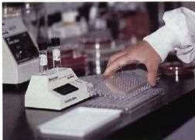
13-12 Broth Microdilution Method—Inoculation of microdilution panel. Microdilution panels are used to quantitatively measure the susceptibility of microorganisms to a battery of antimicrobial agents. The inoculum is mixed and poured into the inoculum/seed tray. The inoculator tips are lowered into the tray and the tips filled by capillary action. The inoculator tips are then lowered into the wells of the panel, as shown here.
