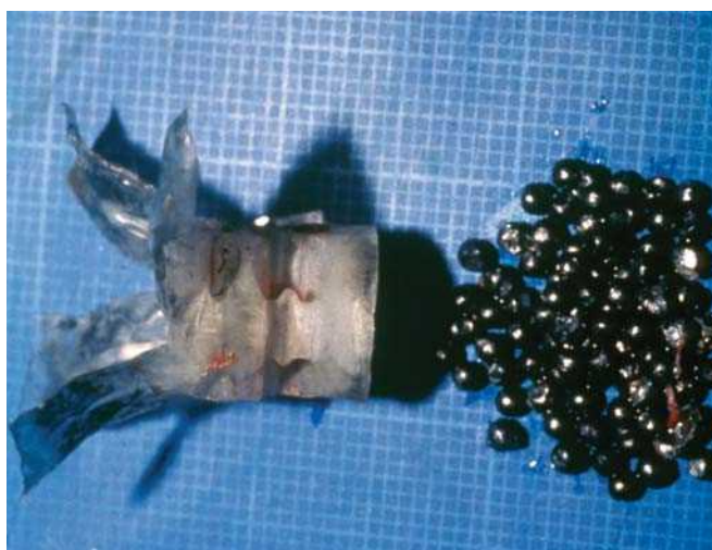
Figure 8.274 Birdshot with power piston-type cup from a shotgun shell.
