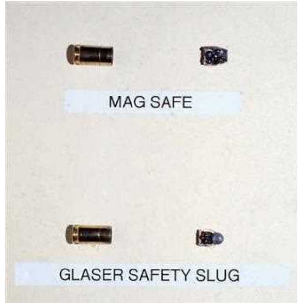
Figure 8.232 This diagram shows a comparison of the components of a Mag-safe ammunition and Glaser safety slug.
