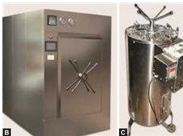
Figs 23.2A to C: Steam sterilizer (autoclave): A. Schematic diagram; B. Horizontal autoclave; C. Vertical autoclave.
