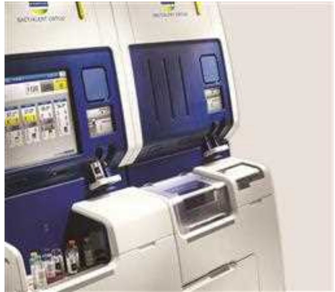
Fig. 3.3.8: BacT/ALERT VIRTUO automated blood culture system.
