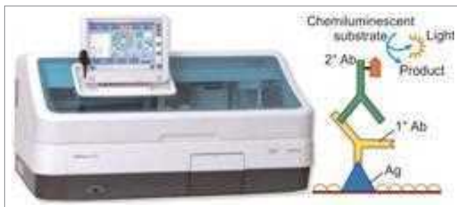
Fig. 12.11: Chemiluminescence system (CLIA) and its principle. Source: Department of Microbiology, JIPMER, Puducherry (with permission).
