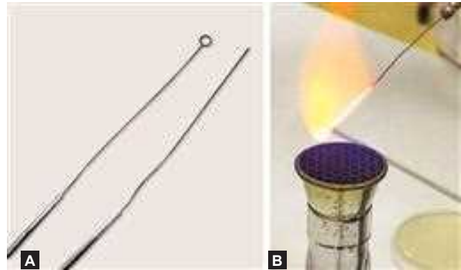
Figs 3.3.9A and B: A. Bacteriological loop and straight wire; B. Flaming the loop (red hot).
