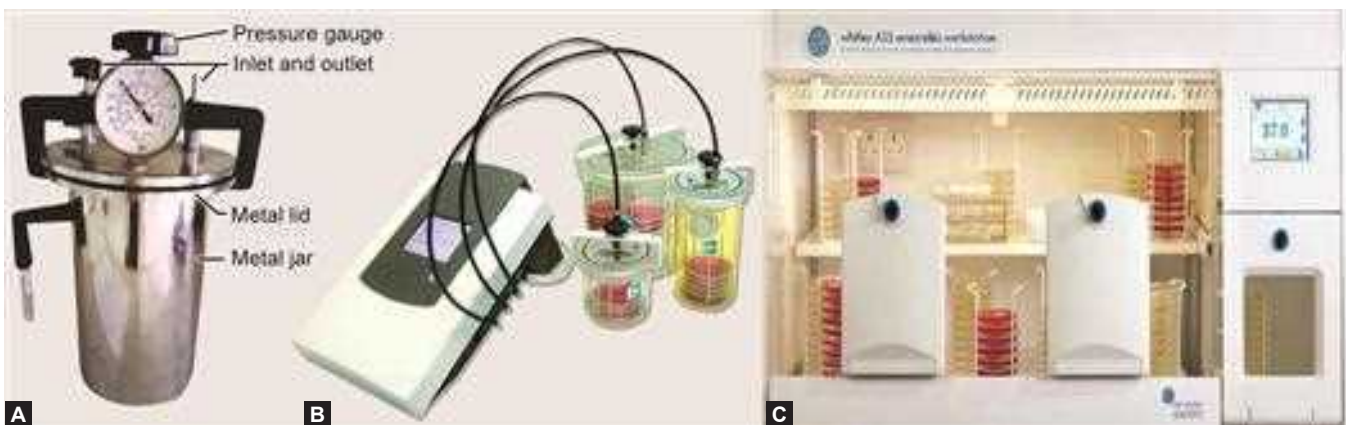
Figs 3.3.15A to C: A. McIntosh and Fildes's anaerobic jar; B. Anoxomat anaerobic system; C. Anaerobic work station (Whitley pvt. Ltd.).
