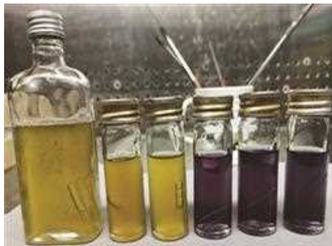
Fig. 27.2: MacConkey purple broth for multiple tube method (one 50 mL and five 10 mL tubes are needed for testing unpolluted water); if negative, media appears purple; if positive, media turn yellow.
