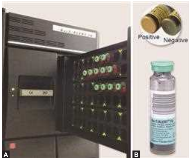
Figs 3.3.7A and B: A. BacT/ALERT automated blood culture system; B. BacT/ALERT blood culture bottle.
