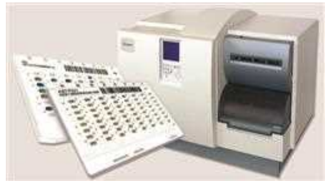
Fig. 3.3.23: VITEK 2 system with its panels (reagent cards) for identification and antimicrobial susceptibility test.
