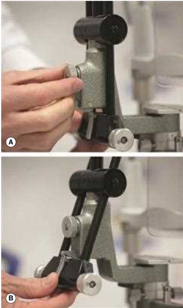
Fig. 1.34 Preparation of the slit lamp for fundus examination. (A) Unlocking the screw; (B) tilting the illumination column
