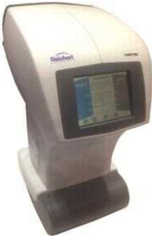
Fig. 1.47 Corneal hysteresis as measured by the Ocular Response Analyzer. It is defined as the difference between the pressure at which the cornea bends inward during air-jet applanation and the pressure at which it bends out again
