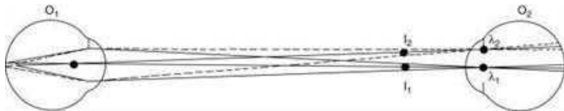
• FIG. 6.4 The course of the emergent rays in myopia of 1 D and at the point of reversal. So long as the light source I_1 is in the pupillary area of O_2 , the pupil of O_1 appears uniformly illuminated and there is no shadow. Directly I_1 passes to I_2 and the light is completely cut off so that the pupil of O_1 becomes completely dark.
