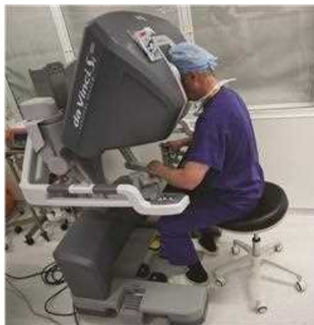
Figure 69.3 The operating surgeon at the console controlling the robotic arms and instruments by the hand cradle.
