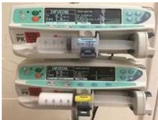
Figure 32.2 Target controlled infusion pumps for propofol and remifentanyl. Pharmacokinetic algorithms calculate drug delivery taking into account patient age, weight and, for remifentanyl, height.
