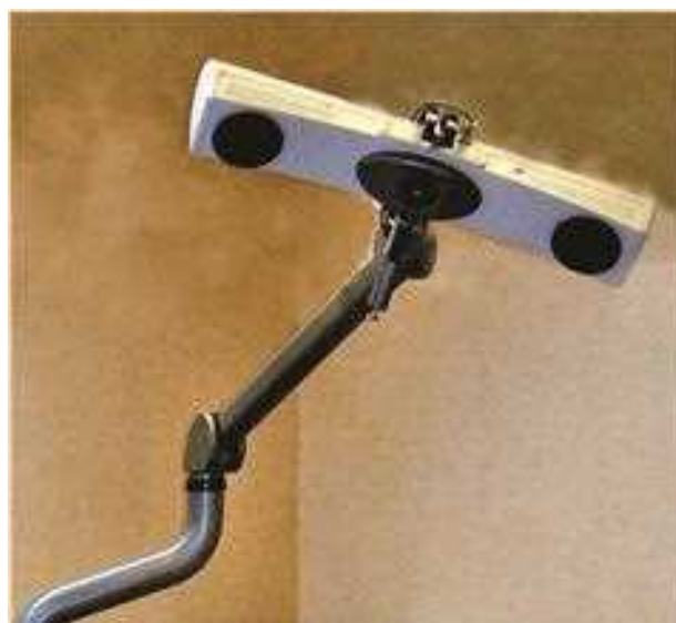
Figure 48.6 An infrared optical tracking system. In the centre of the gantry is a laser light that is used to position the arm during the set-up procedure.
