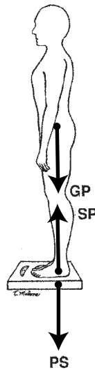
Figure 1-29 Although a scale is commonly thought to measure the weight of the person (gravity-on-person [GP]), it actually measures the contact of the person-on-scale (PS). Vectors GP and PS are equal in magnitude as long as nothing else is touching the person.
