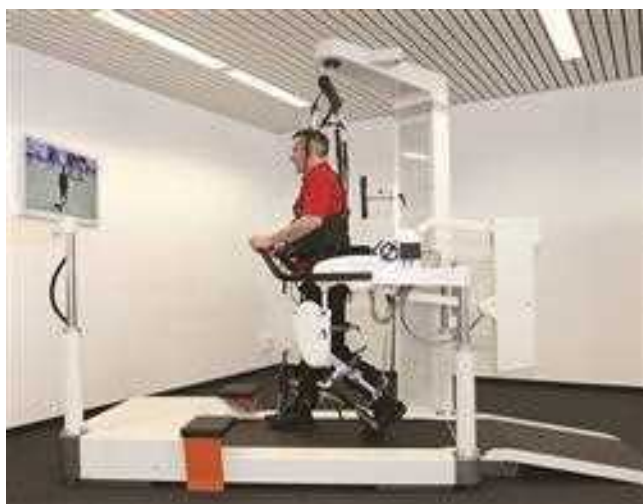
Fig. 38.2 Body weight–support trainer or body weight supported treadmill trainer: Lokomat robotic system. (Courtesy Hocoma, Volketswil, Switzerland.)
