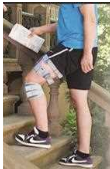
Fig. 14.58 Bioness L300 system is a neuroprosthetic device that contains an orthotic cuff and electrodes. It fits just below the knee to supply FES to the lower leg, targeting the peroneal nerve to cause dorsiflexion. An additional thigh cuff (L300 Plus) can be added to help assist with knee flexion and extension and provide additional support. Courtesy of Bioness, Inc.
