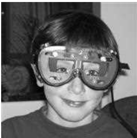
Fig. 28.14 The Visagraph (boy with goggles) measures eye movement while the subject is reading.
