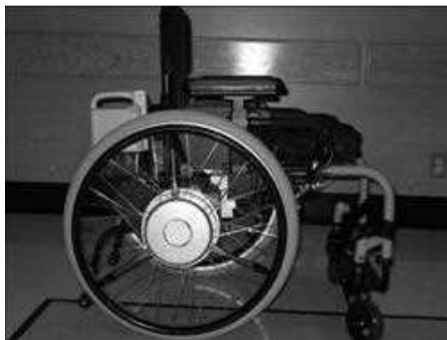
Fig. 14.63 Power assist wheels added to a manual wheelchair meet the needs of users who may need supplemental support in the community while also requiring the ease of transportation that a manual chair provides. Power assist wheels help users with energy conservation and shoulder maintenance long term.
