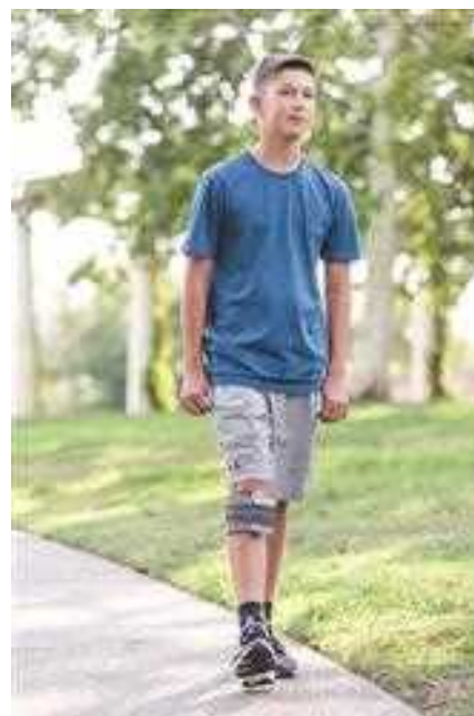
Fig. 14.59 The WalkAide System is a neuroprosthetic device that contains an orthotic cuff and electrodes. It fits just below the knee to supply functional electrical stimulation (FES) to the lower leg, stimulating the appropriate muscles and causing dorsiflexion. It is activated by a tilt sensor mechanism and relies on the angle of the tibia for appropriate timing of the FES to assist with foot drop. Courtesy of Hanger, Inc.
