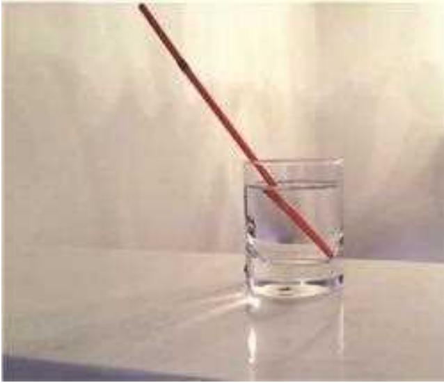
Fig. 28.2 Refraction: Bending of Light at Air-Water Interface. (From Khalili K. Diagnostic Ultrasound . Elsevier: Philadelphia; 2018.)
