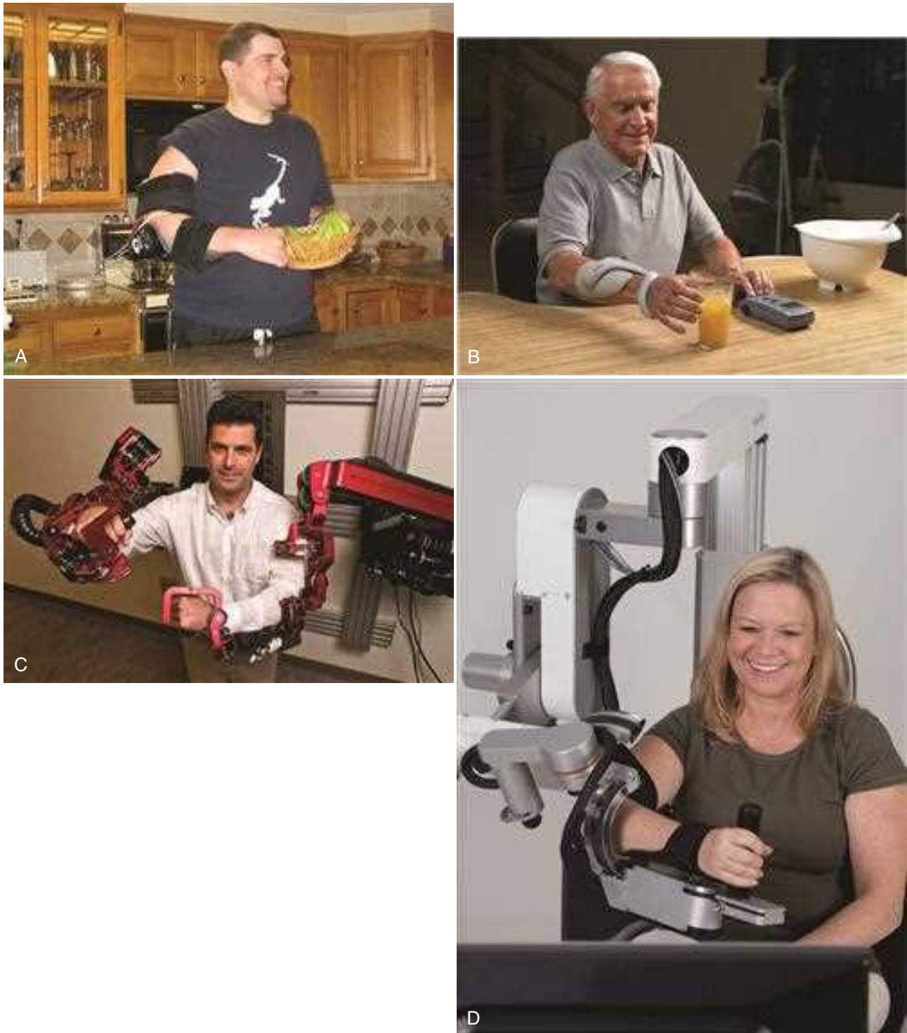
Fig. 38.3 Wearable Upper-Limb Devices and Assistive Robotic Exoskeleton Devices. (A) Myomo upper-limb robotic assistive device. (B) Bioness L200 arm and wrist trainer. (C) Shoulder, elbow, and wrist upper-limb assistive robotic bilateral device. (D) Armeo robotic arm. (A, Courtesy Myomo, Cambridge, MA. B, Courtesy Bioness, Valencia, CA. C, Courtesy Jacob Rosen/Jim Mackenzie, UCSC. D, Courtesy Hocoma, Volketswil, Switzerland.)
