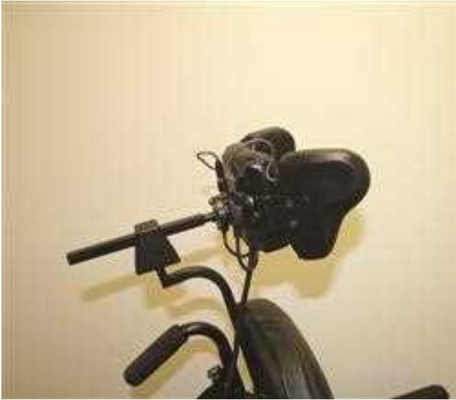
Fig. 14.42 Head array is a headrest and head control for driving wherein the position of the head activates the drive control of the wheelchair. It is appropriate for persons with high cervical injuries. The head array switches can be adjusted to the individual's specific needs relative to their active range of motion and control of their head. The switches are embedded in the headrest panels and not only control driving but can also control the activation of other devices for environmental control. The side panels of the headrest can be straight or curbed depending on the needs of the patient. Additionally, the head array can be sized for either adult or pediatric patient.
