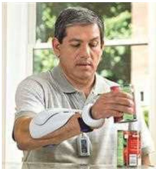
Fig. 14.61 The Bioness H200 system is a neuroprosthetic device that contains an orthosis for the upper extremity and electrodes. It fits to the wrist and forearm and targets opening and closing of the hand and fingers. The device can be used in an exercise mode or to perform functional tasks. Courtesy of Bioness, Inc.
