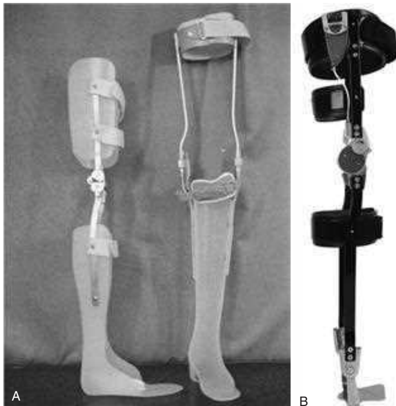
Figure 16-52 ■ A , Polypropylene knee-ankle-foot orthosis (KAFO) and combination plastic and metal KAFO. B , Stance-control KAFO knee joint. This joint combines the stability of a locked knee during the stance phase of walking but allows flexion of the limb for the swing phase of gait. A locked knee makes it much harder to clear the leg over the ground. Some long leg brace users are perfect candidates for the stance-control KAFOs. These devices, through a few different types of joint mechanisms, create a locked knee when the leg is supporting the weight of the body but unlock when the leg is lifted to allow for easy advancement of the leg as it is allowed to bend. For the right patients, this allows them as much mobility to get around as it does stability.
