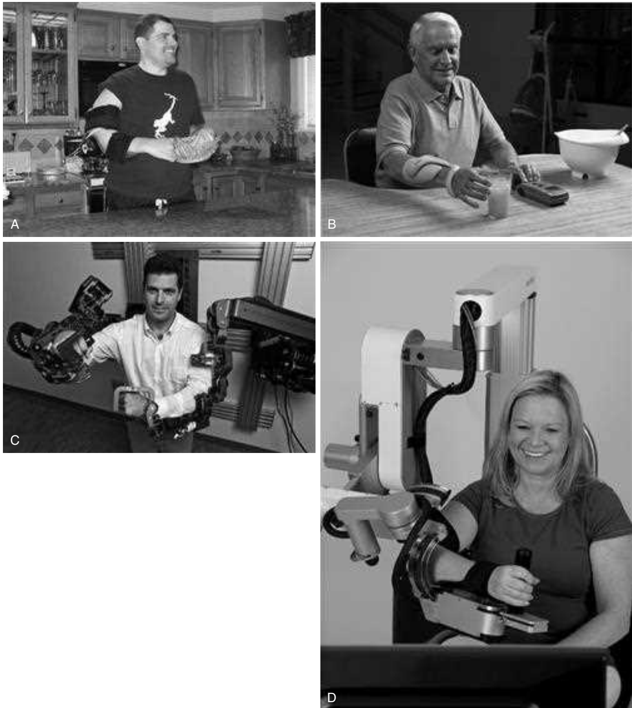
Figure 38-7 ■ Wearable upper-limb assistive robotic exoskeleton devices. A , Myomo upper-limb robotic assistive device. B , Bioness L200 arm and wrist trainer. C , Shoulder, elbow, and wrist upper-limb assistive robotic bilateral device. D , Armeo robotic arm. ( A , courtesy Myomo, Cambridge, Mass; B , courtesy Bioness, Valencia, Calif; C , courtesy Jacob Rosen/Jim Mackenzie, UCSC; D , courtesy Hocoma, Volketswil, Switzerland.)
