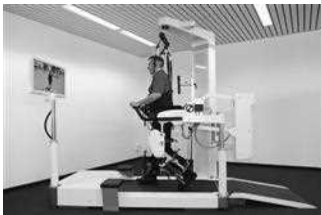
Figure 38-3 ■ Body-weight–support trainer or body-weight–supported treadmill trainer: Lokomat robotic system. (Courtesy Hocoma, Volketswil, Switzerland.)
