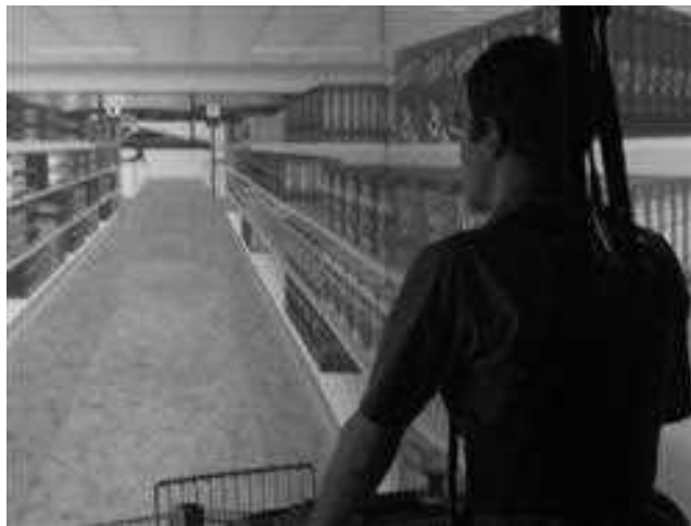
Figure 38-10 ■ The Balance Near Automatic Virtual Environment (BNAVE). A patient walking on the treadmill through the virtual grocery store while pushing a cart. The vest was worn to ensure safety.
