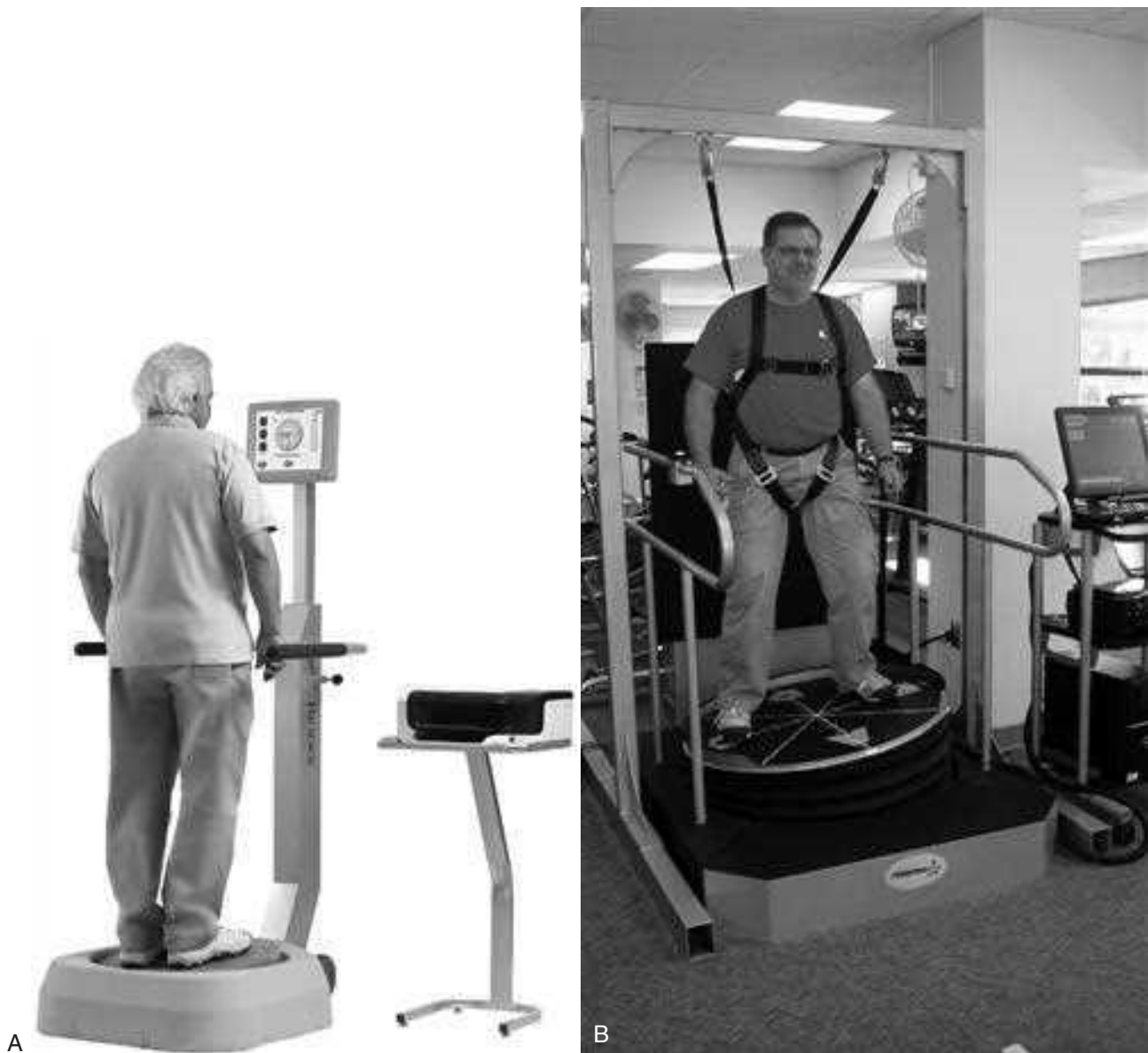
Figure 22-21 ■ Advanced technology to support balance and gait retraining. Other systems provide surfaces that can be made unstable ( A ) or made to move ( B ). The surface motion provides both biomechanical and somatosensory challenges. Amplitude and velocity capacity also vary from system to system. Both systems shown here provide omnidirectional motion. A , Biodex Balance System SD measures the motion on the surface, B , Proprio Reactive Balance System uses motion sensors on the body placed at the level of the COG ( A , Courtesy Biodex Medical Systems, Shirley, NY; B , Courtesy Perry Dynamics, Decatur, Ill.)
