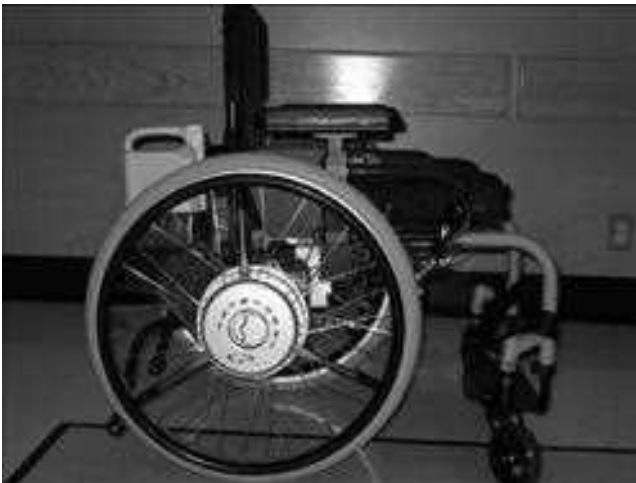
Figure 16-45 ■ Power assist system. The Xtender by Sunrise Medical is one of three power assist systems available. The motors are in the wheels. The battery extends off the back of the wheelchair. There is a connection between the motors in the wheels. The system is added to a manual wheelchair. There are two power assist levels.
