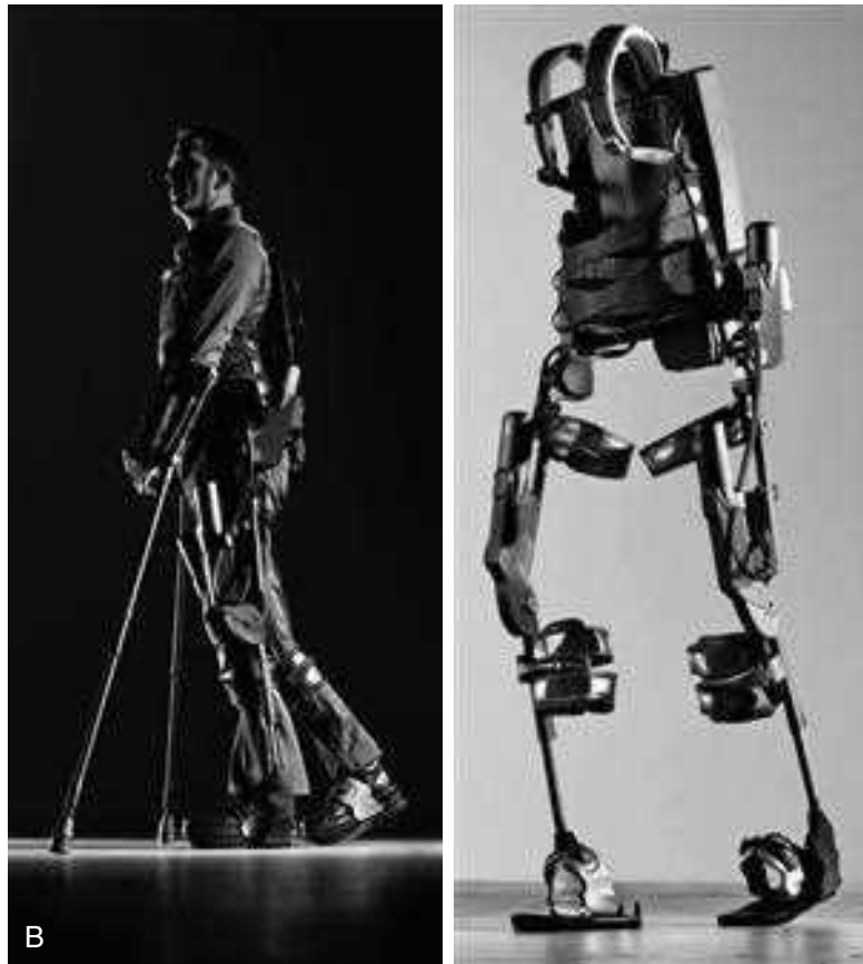
Figure 38-8 ■ Lower-limb robotic assistive devices (with and without NES). A , Tibion Bionic Leg. B , Ekso Bionics bilateral wearable lower-limb assistive device. (A, courtesy Tibion, Sunnyvale, Calif; B, courtesy Ekso Bionics, Richmond, Calif.)
