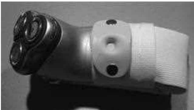
Figure 16-23 ■ Simple razor adaptation that helps turn razor on and off with a grosser motor movement.
