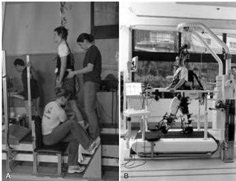
Figure 16-60 ■ A , Manual treadmill. Treadmill training with body-weight–supported and manual assistance is being completed on the TheraStride Innoventor, which combines a treadmill and support harness system with software that measures variables of gait training, including speed, weight supported, and amount of time walked. Two or three therapists are needed to provide assistance at the trunk and lower limbs to facilitate an appropriate gait pattern. B , Robotic treadmill. The Lokomat by Hocoma is a robotic-assisted treadmill that provides adjustable body-weight support and gives clinicians the ability to adjust gait-specific parameters when completing training with patients who have mobility deficits.
