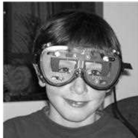
Figure 28-14 ■ The Visagraph (boy with goggles) measures eye movement while the subject is reading.
