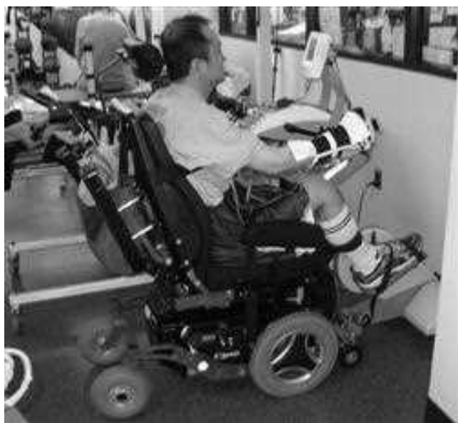
Figure 16-65 ■ RT300 SA Arm system is a functional electrical stimulation (FES) upper body ergometer designed to stimulate muscles of the upper extremities. Adhesive electrodes can be applied to a variety of muscle groups over the trunk, shoulders, and arm muscles and are stimulated at the appropriate time to facilitate a cycling motion using the upper-extremity ergometer. FES bike software has the capability to store patient-specific parameters between sessions and clients.
