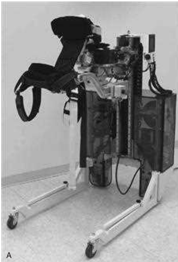
Figure 38-6 ■ KineAssist gait trainer–destabilizer. (Courtesy Kinea Design, Evanston, Ill.)
