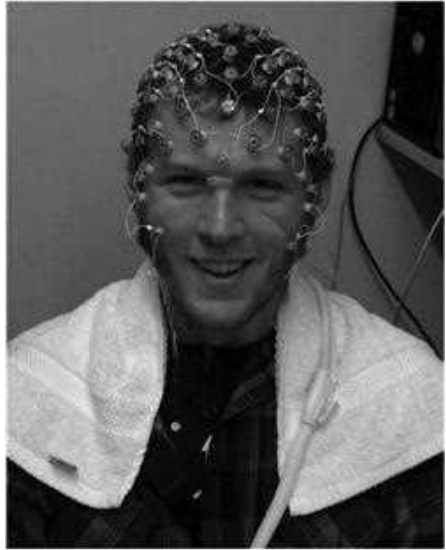
Figure 38-17 ■ A subject with an electroencephalogram net placed on his scalp for a research experiment. There is some variability in the placement of the net, which may affect the calibration required each time the net is placed.
