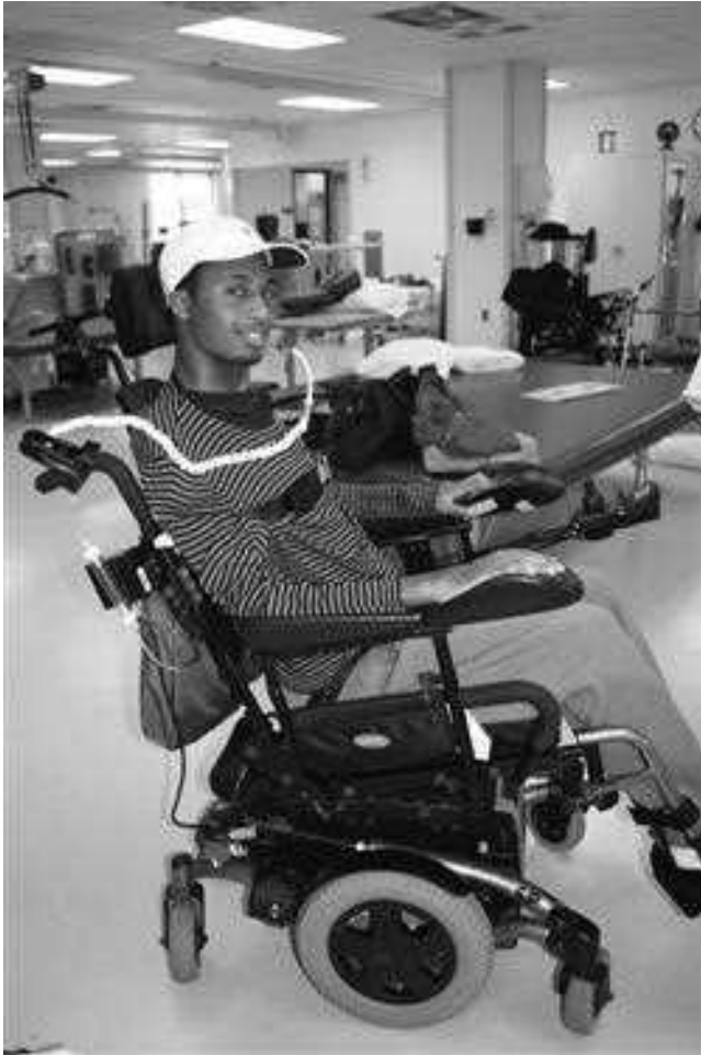
Figure 16-36 ■ The pneumatic control (sip-and-puff straw) is usually ordered on a power reclining or tilt-in-space wheelchair for patients with injury levels above C6. The straw is removable, and several are supplied with the wheelchair. The straw is attached to a flexible arm, and it is adjustable to different heights and angles to fit the needs of the patient.
