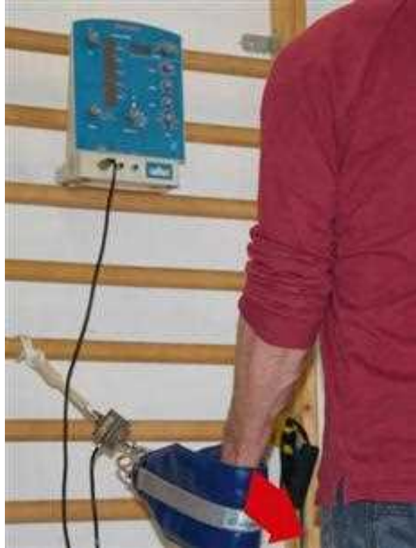
Fig. 3.38 Exercise for the ulnar stabilizers of the wrist with load cell and visual feedback
