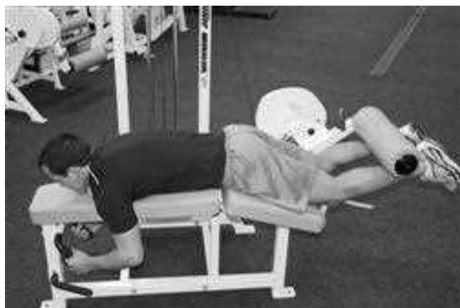
FIGURE 6.48 Variable resistance by means of a cam mechanism in the weight-pulley system is applied to concentric and eccentric contractions of the hamstrings as the knees flex and extend.
