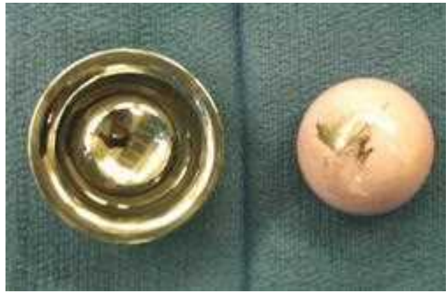
Figure 43-13. Failed ceramic on metal hip arthroplasty components. Note the metallic staining on the ceramic femoral head.
