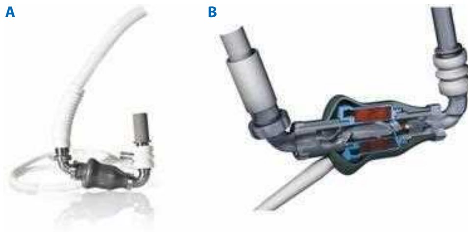
Figure 21-12. The HeartMate II LVAD viewed from the (A) outside and (B) inside. The device is an axial flow, rotary pump that produces no pulsatile action. The pump contains a magnet, and the rotor assembly functions by the electromotive force generated by the motor. The result is that blood is propelled from the inflow cannula to systemic circulation at flows up to 10 L/min. (Images reprinted with the permission of Thoratec Corporation.)
