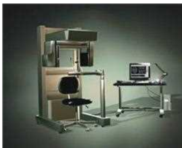
Figure 18-5. POC-CT system. All components can be fit within an 8' × 10' room in an outpatient office setting.
