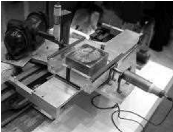
Fig. 7. Hounsfield's prototype for the CT scanner. Note the section of brain in the centre of the image. Image by courtesy of Philip Cosson.
