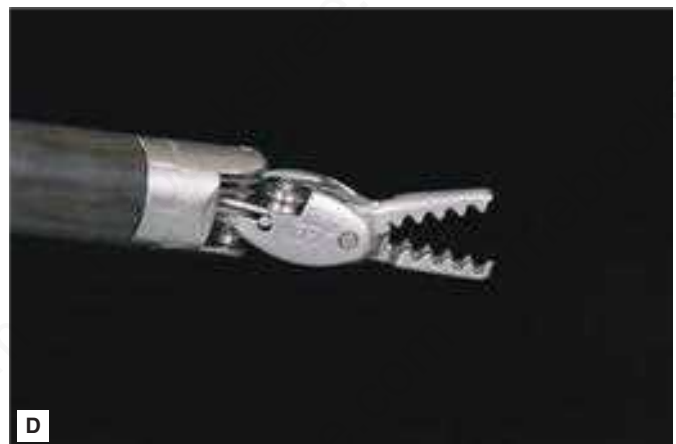
FIGURE 40-23 Robot-assisted mitral valve surgery: end-effector instruments. (A) Suture-cut needle holder; (B) large needle holder; (C) curved scissors; and (D) Resano forceps.
