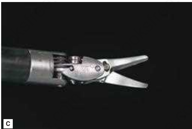
FIGURE 40-23 Robot-assisted mitral valve surgery: end-effector instruments. (A) Suture-cut needle holder; (B) large needle holder; (C) curved scissors; and (D) Resano forceps.
