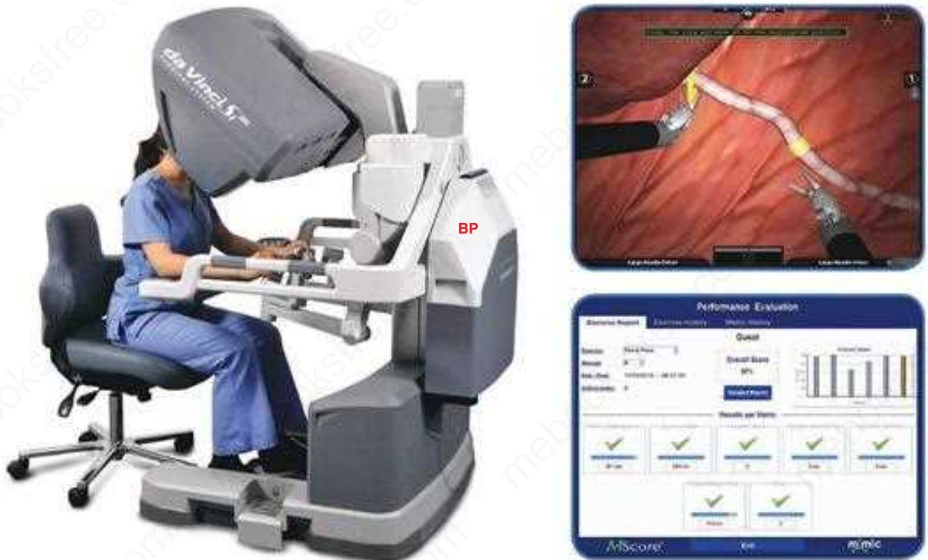
FIGURE 40-21 Robotic simulation: da Vinci Skills Simulator. The “Backpack” (BP) Skills Simulator attaches directly to either a daVinci SI or XI surgeon console. Various surgical simulated tasks challenge the surgeon and a report is generated. With advancing skills more difficult tasks are provided. (Used with permission from Intuitive Surgical Inc., Sunnyvale CA.)
