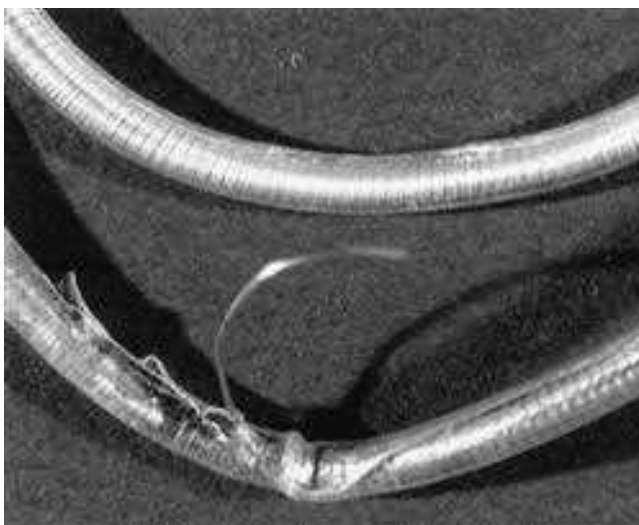
FIGURE 55-20 Telectronics Accufix atrial J-leads removed for retention wire fracture. Region of fracture appears benign in upper image. Lower image illustrates retention wire extrusion after percutaneous extraction. Extruded wire resembles a safety pin.
