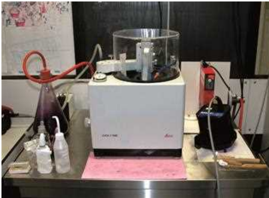
Figure AIII-4. The Leica SP1600 microtome uses a diamond-coated inner-hole saw blade.
