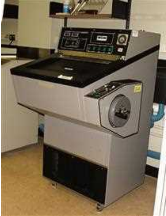
Figure All-5. Freezing microtome (cryostat for sectioning frozen tissue).
