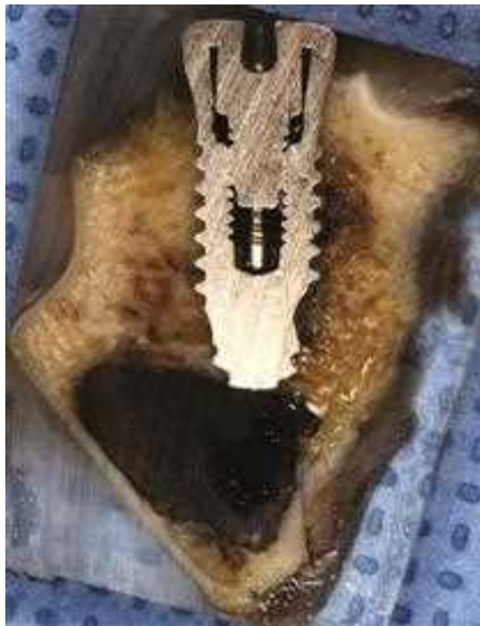
Figure All-6. A dental Implant embedded in methyl methacrylate (MMA) in rabbit femur during the sectioning.
