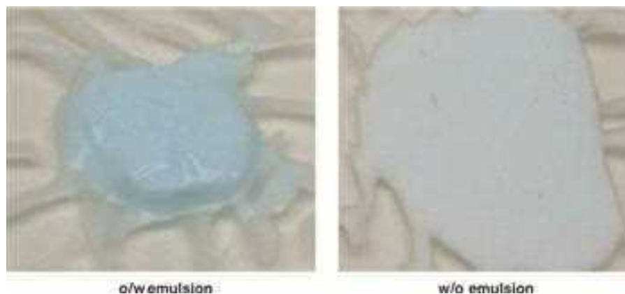
Figure 33.2 Both emulsion types are intensely opaque with differing degrees of reflectance. Equal amounts of water-soluble dye and base were used to create the image. The oil-in-water (o/w) emulsion has a continuous phase of water and the dye imparts the color to this phase (darker intensity). The water-in-oil (w/o) emulsion is less intense in color since color is restricted to the discontinuous or suspended phase.
