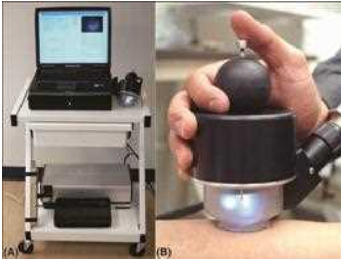
Figure 53.8 The DermaCorder™, a commercially available vibrating probe device, was used to measure wound electric potential by Nuccitelli et al. to investigate the effect of age on wound electric potentials in human subjects. Source: From Ref. 30.
